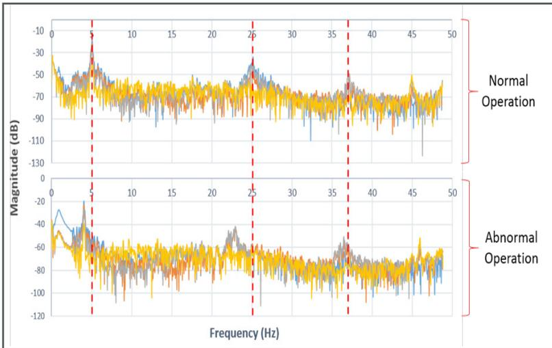
The graph above shows the data that was sent to ThingWorx. It was used to identify when the frequencies deviated from the location associated with normal operation.
