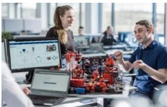
*Image 1: The compact fischertechnik Training Factory Industry 4.0 illustrates the processes of a digitalised factory.*
