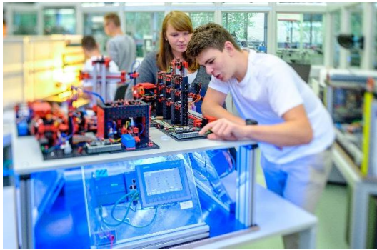
Image 1: The fischertechnik Training Factory Industry 4.0 24 V can be used to realistically simulate real and digital processes in a smart factory.
