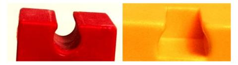
These fit snuggly together. The pins are designed to enter at a 90 degree angle and not allow the part to rotate.
