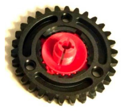
The cap is lightly placed on the axle and the entire assemble is slid into position and tightened. To adjust you will need to loosen the nut and then retighten the cap when it is exactly where you want it.
