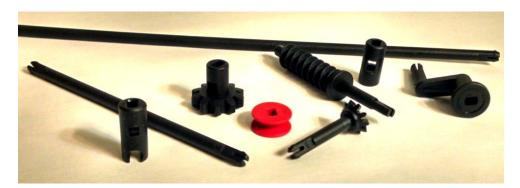
The special shape on the end allows the part to compress when entering the other component and then expand holding it firmly in place. The picture below shows the clip axle end on the bevel gear and the clip axle receptor on the cog wheel. The bevel gear is aligned and then slowly inserted into the cog wheel until a small click is heard. The remove the parts the force is directly reversed with a smooth pulling action to separate the components.
