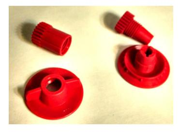
They consist of a threaded part that has separations in it. As the tapered cap is threaded onto the collet the sections of the collet squeeze together and clamp onto the shaft passing through the center. When the collet is loose the shaft is free to pass in and out. When the cap is tightened the movement ends and the shaft is caught in position. In the example below a collet is used to hold a gear in position on a shaft.
