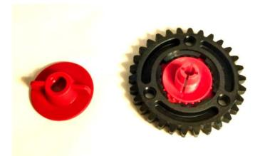
Notice the collet has notches on the outside to help the gear connect with the collet.
