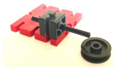
There are also times when we want to use objects besides a pulley on an axle. Hubs are used to allow soft objects such as tires to be utilized with the specially sized axles. The hubs are designed to push into the center of the tire and the friction fit keeps them aligned.
