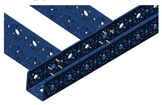
Using the 2mm hex key, screw the M3 x 10mm BHCS through the 432mm U-Channel into the tapped holes of the end piece plates of the two assemblies completed in step 1.
