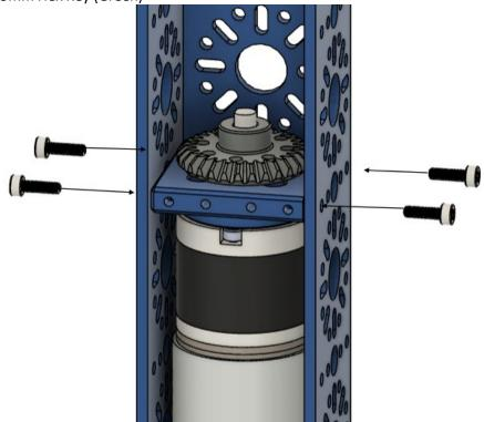
Screw the orbital mount into the 288mm U-Channel using four, M3 x 10mm SHCS.
