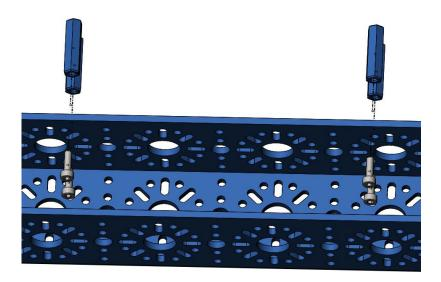
On the middle 192mm U-Channel, attach  $4 \times M3 \times 10$ mm SHCS and  $4 \times 25$ mm Standoffs. The standoffs should be facing the omni wheels.
