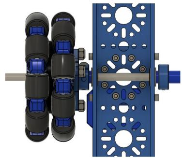
Using the screws, screw in the arm and oms to the drive base. Repeat on the other side.
