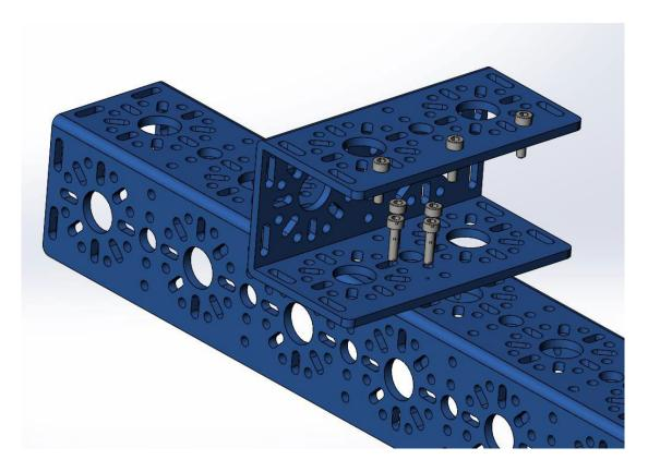
Screw the 96mm U-Channel into the 384mm U-Channel. The Small 8mm hole should line up with the third small 8mm hole from the end of the 384mm U-Channel.
