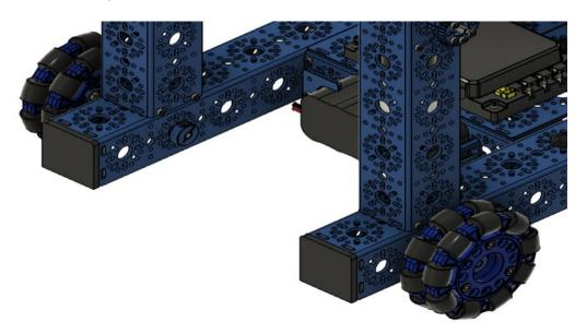
Line up the ARM and OMS with the drive base. The 2, 288 U-Channels should be over the shafts of the omni wheels.
