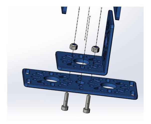
Screw a 96mm x 40mm flat into an inside L bracket.
