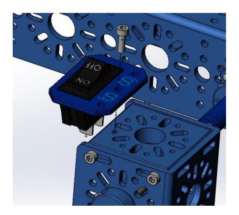
Screw the On/Off switch into the end piece plate.
