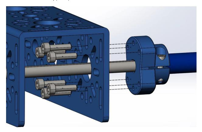
Using the M3 screws, screw the 384mm U-Channel into the clamping shaft hub.
