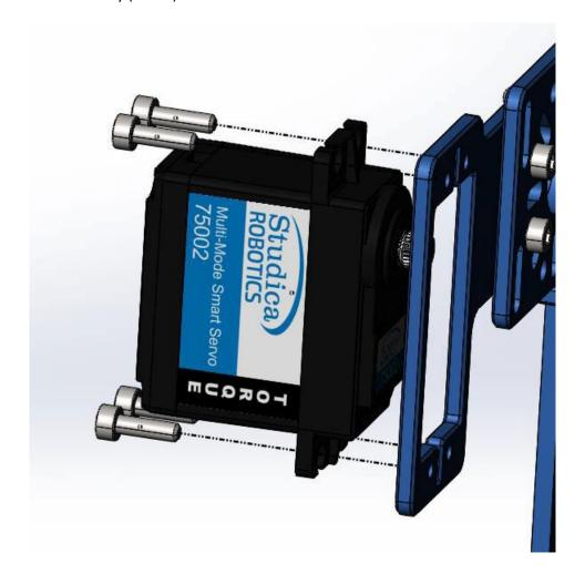
Screw the servo into the servo bracket.
