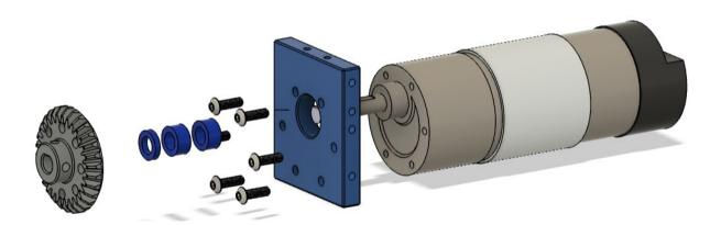
Slide the motor into the motor mount plate and use the 6 x M3 x 10mm BHCS to tighten the motor onto the plate. Slide the four spacers and the bevel gear onto the motor shaft. **NOTE: THE SPACERS AND GEARS WILL BE LOOSE.**
