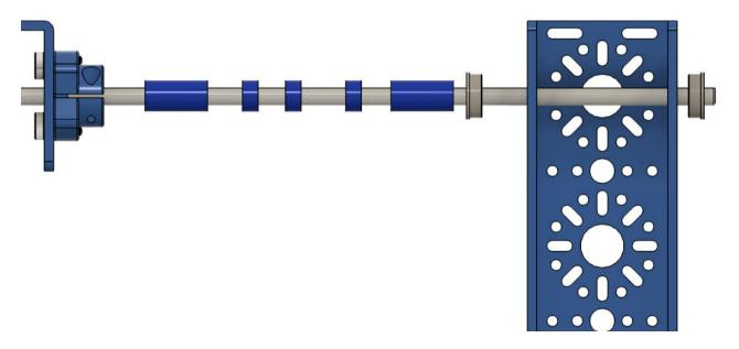
Slide the spacers, bearing and U-Channel together as shown.
