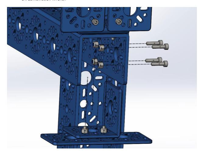
Screw the assembly from step 16 into the 384mm U-Channel.
