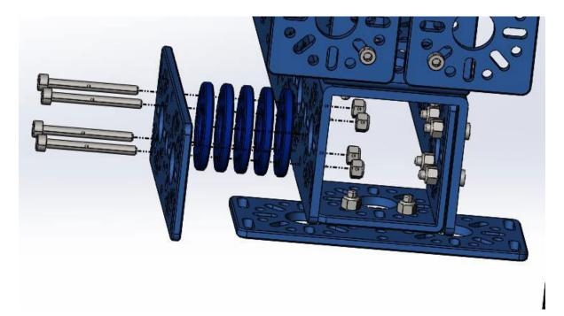
Slide the screws through the 96mm flat and five pattern spacers into the 384mm U-Channel. Lock them in place with Nyloc nuts.
