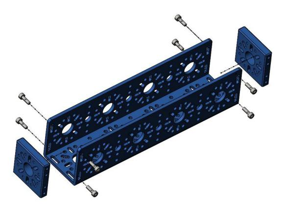
Using the Green 2.5mm Hex key screw  $4 \times M3 \times 10$ mm SHCS into the end piece through the holes of the 192mm U-Channel. Note the end piece plate must sit flush with the ends of the 192mm U-Channel.
