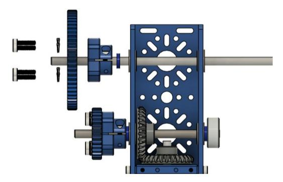
Attach the 64-tooth gear to the clamping shaft hub just as we did in the previous step with the 32-tooth gear. Slide the shaft hub, a spacer, and a bearing onto the 432mm U-Channel. Place the other bearing on the other side of the channel and slide the shaft through. Do not tighten the shaft hub yet.
