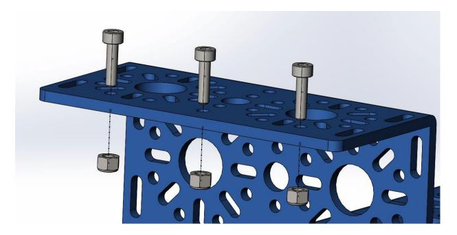
Screw the three screws into the 96mm U-Channel while using Nyloc nuts to keep them tight and locked in.
