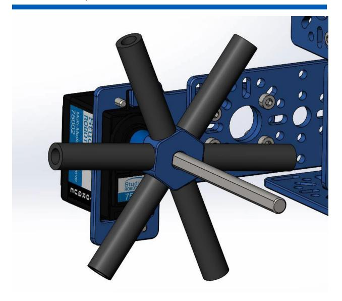
Slide the tubing onto the spokes and lock it into place with a zip tie at the ends.
