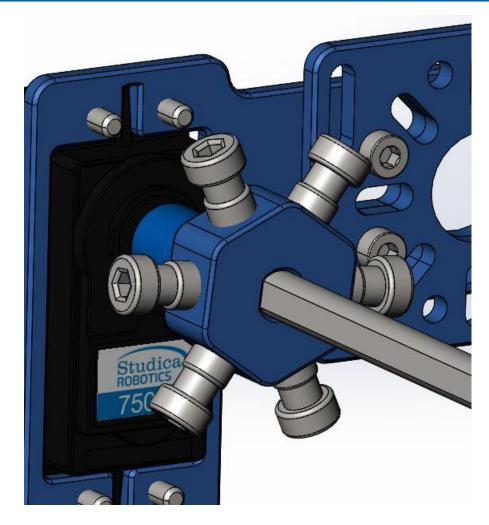
Insert the spokes and tighten down. Cut 6 x 25mm length strips of the rubber tube.
