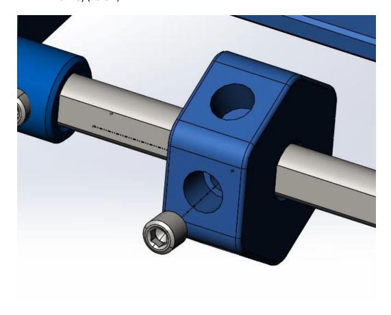
Slide the intake hub down the shaft to the servo hub and tighten it down.
