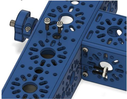
Screw in the final four, M3 x 10mm SHCS. Repeat this step for the other side.
