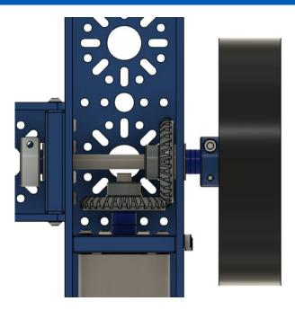
The gears should have a good mesh and not be loose.
