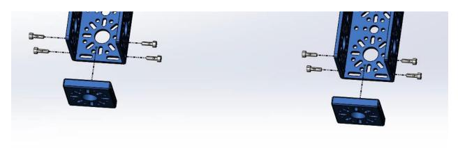
Screw end piece plates into the bottoms of the two 288mm U-Channels.
