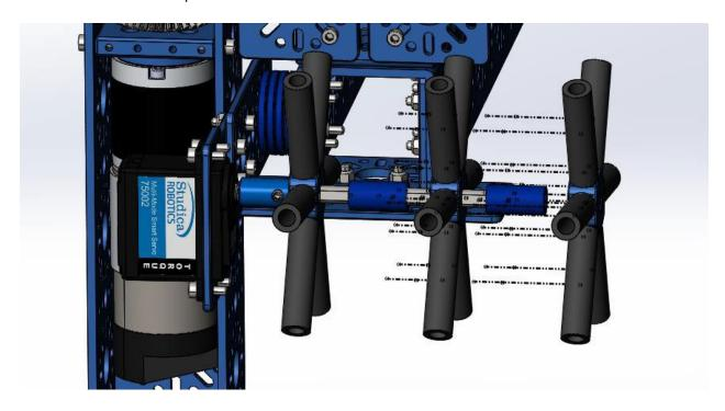
Repeat step 21, 2 times to create two more intakes. Use a 20mm spacer to separate the intakes on the shaft.
