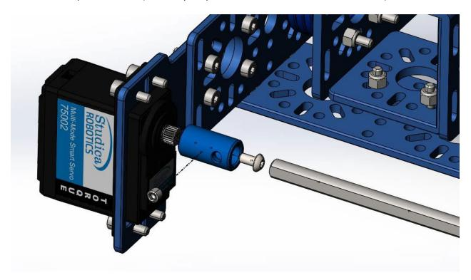
Slide the 25T to 6mm hub onto the servo's output shaft. Using the BHCS, screw the hub into the servo. Slide the D-Shaft into the hub and tighten it down with the set screw.
