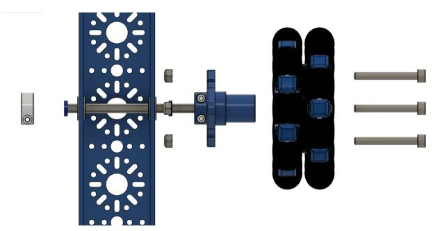
Start by placing the enhanced wheel hub (triangle piece) into the Omni wheel. Take out three shorter M5 screws inside the enhanced wheel hub kit. Slide the screws through the wheel and the hub. On the other end of the hub, use the M5 Nyloc Nuts to secure the screws to the hub. You will need the Yellow 4mm hex key and the 8mm wrench to tighten the nuts fully.
