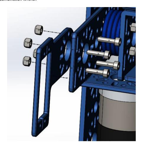
Screw the offset plate into the 96mm flat.
