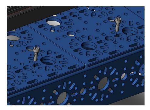
Screw the other end of the 192mm x 96mm flats into the 192mm U-Channel using two, M3 x 12mm SHCS.
