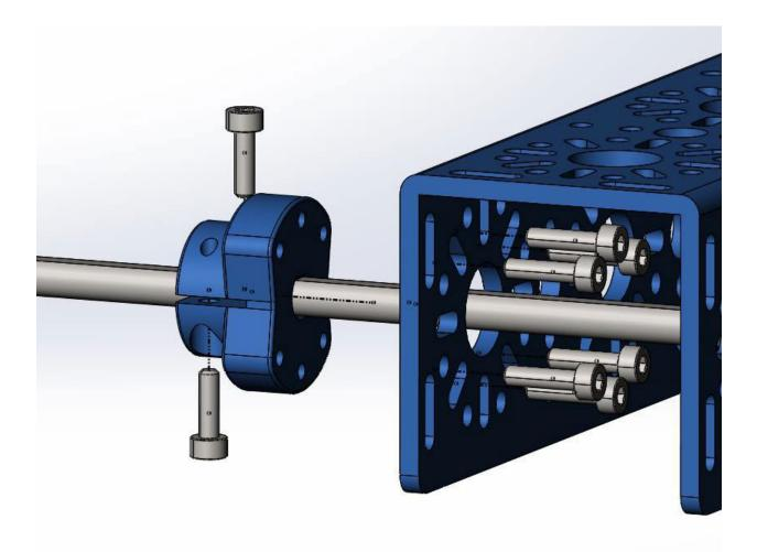
Slide the clamping shaft hub from the other side of the shaft and screw it into the 384mm U-Channel.
