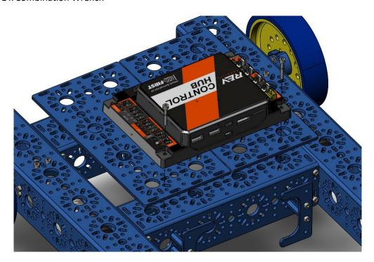
Using the two, M3 x 20mm SHCS, screw the Control Hub through the 2, 192mm x 96mm flats into the 192mm U-Channel of the drive base.
