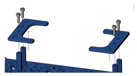
Screw the battery clips into the four standoffs using the last 4 M3 x 10mm SHCS.
