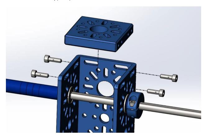
At the top of the 288mm U-Channel, screw in an end piece plate.
