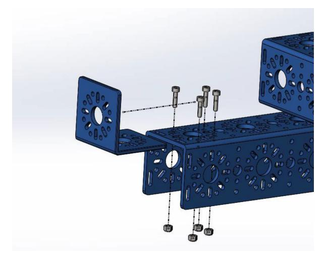
Screw the L bracket to the end of the 384mm U-Channel using four, M3 x 12mm SHCS with Nyloc Nuts.
