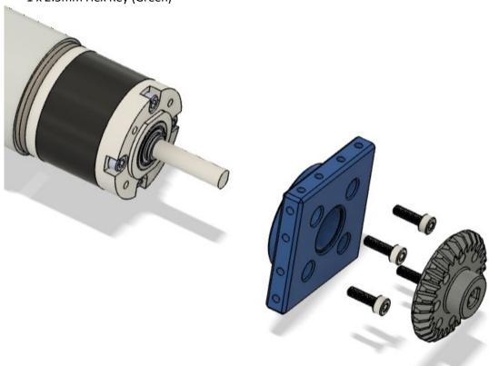
Slide the motor onto the orbital mount and screw it in using the M3 x 10mm SHCS. Slide the bearing into the bearing hole of the orbital mount and then slide the spacers and the bevel gear on top.
