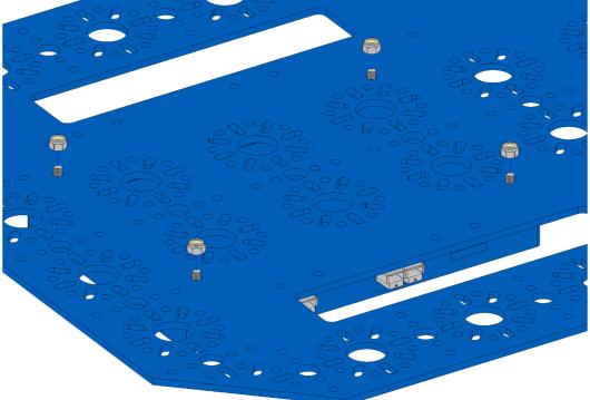
Using 4 M3 x 12mm Screws and 4 M3 Nylock nuts, secure the VMX to the base plate from the previous step.
