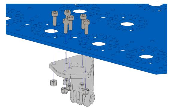
Using an M5 x 20mm screw and an M5 nut, secure the other half of the camera mount.
