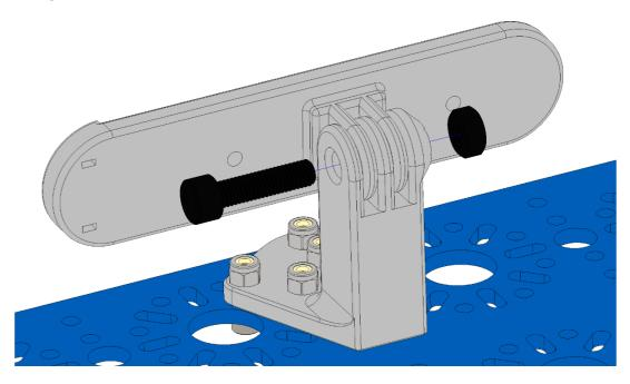
Attach the depth camera with 2 M3 x 8mm screws.
