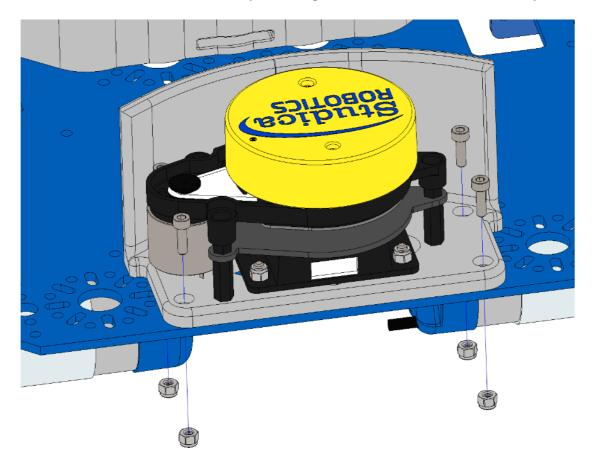
Attach the LIDAR mount to the baseplate using 4 M3 x 12 mm screws and 4 M3 Nylock nuts.
