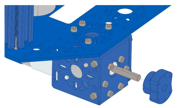
Insert an M3 x 25mm screw through the Mecanum Wheel and screw it into the clamping hub. Repeat this step 5 times for the remaining screws. Repeat Step 8 for all the remaining wheels. Please see next page for important diagram of proper wheel alignment.
