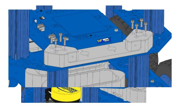
On the other side, put the screws through the control panel mount.
