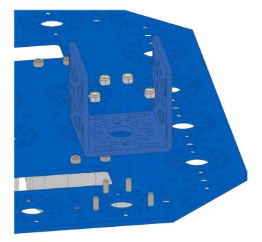
Attach the Maverick Motor to the motor mount plate using 6 M# x 12mm Screws.
