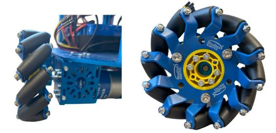
IMPORTANT NOTE: The rollers of each wheel should be pointed inward towards the wheel diagonal to it to form an "X" Shape (See image above for reference). (Back Left Wheel pointing towards the Front Right Wheel, and Back Right Wheel pointing towards the Front Left Wheel)
