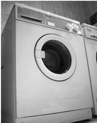
■ The most widespread design is the drum washing machine, in which a washing drum rotates around an axis. The advantage of this machine type is the small size so that, for example, it can be installed in kitchen units.
