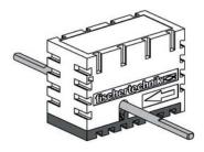
What happens in the motor? The motor consists of gear, a wound-up spring, shafts and a housing. The spring is permanently connected to the housing and to a shaft over the gear. The spring is tensioned in the same manner as winding up a clock. When the vehicle is released the spring unwinds, transferring the stored energy to the
