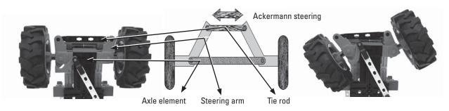
The steering wheel is connected to the tie rod by a rack and pinion. When you turn the steering wheel in one direction, the steering arms turn the wheels as well as the axle in this direction. Due to the trapezoidal layout the outer wheel moves through a larger arc then the inner wheel, making the cornering more precise.
