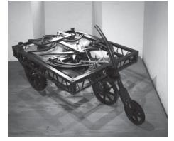
■ "What does Leonardo da Vinci have to do with a pullback motor? In his sketches he left a model of a three-wheeled vehicle. This motor consisted of components such as wooden springs and gears. The springs were tensioned by muscular force. The energy stored in the springs was then transferred to the drive wheels when a catch was released.
