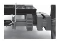
For this purpose thread the blue string through the opening provided for this purpose in the axle. Pulling the vehicle back, winds the string around the axle, tensioning the flexible spring. When the vehicle is released, the bending rod returns to its vertical position. The string is unwound from the axle, causing the vehicle to move.
