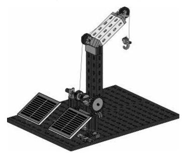
A load should be lifted using solar energy with this model. The trick with antiparallel connection is that the motor does not move as long as both solar cells are lit equally bright. If you cover one solar cell, the motor moves in one direction; if you cover the second cell, it moves in the other direction. In this way, you can replace a pole-reversing switch with two solar cells.
