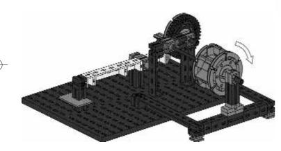
You can hold the waterwheel under a water faucet. Note the direction of rotation of the wheel given in the assembly instructions.
