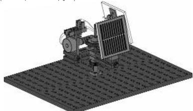
This simple device makes it possible for the solar cells to "move along with" the sun and orient themselves like a compass to the sun. The "tip" where the two solar cells meet always points in the direction of the sun. Pay attention during assembly to the correct connection of the cable, because otherwise the model might move away from the sun instead of to it.
