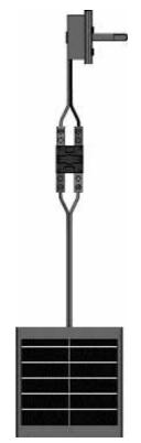
The solar cell provides 0.6 V and a maximum current of approx. 930 mA. The motor has a rated voltage of 2 V, but it already starts to rotate starting form 0.3 V (idling, i.e., without necessity of model driving the motor shaft). Consequently, it can be run with one single solar cell.
