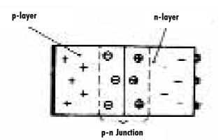
The more light (i.e., energy) that hits the cell, the "more movable" the electrons become; in other words, they can migrate farther. When we connect a solar cell to a consumer (motor, lamp or similar device), they move preferentially in this direction (this can be imagined as a suction effect). Because we can imagine a current flow as a cycle, electrons move repeatedly to the n-layer and migrate again to the p-layer. This flow of electrons results in the current flowing, i.e., the motor rotates.
