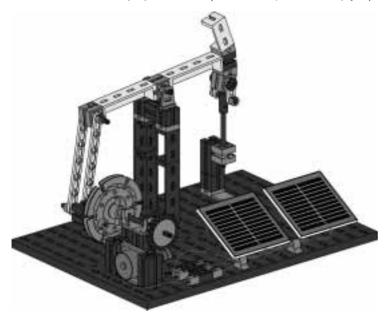
Using such an oil pump, for example, you can pump oil from deep below the earth in desert regions where the sun shines continuously. To drive this model, the motor needs a rather high starting voltage for it to rotate at all. Consequently, two solar cells are connected in a series, as described in the assembly instructions. As a result, the voltages of the two solar cells are added together.
