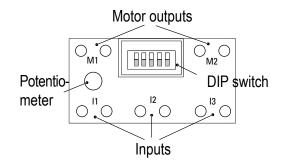
The ROBOTICS module works only when it is connected to a 9 V power supply. For this pur-
