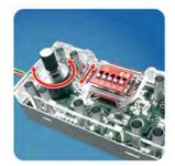
The potentiometer on the ROBOTICS module allows you to control the speed of the two drive motors. When the potentiometer is in the middle position (viewed from above, so that the DIP switch designation is easily legible) both drive motors turn at the same speed propelling the Mini Bot straight ahead. Turning the potentiometer to the left causes it to curve to the left while moving forwards. Turning the potentiometer to the right causes it to curve to the right while moving forwards.
